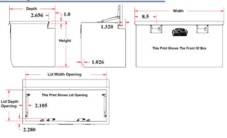
Note: Toolboxes less than 48 inches wide come standard with one lock only; however, we can make configuration changes if specified.
