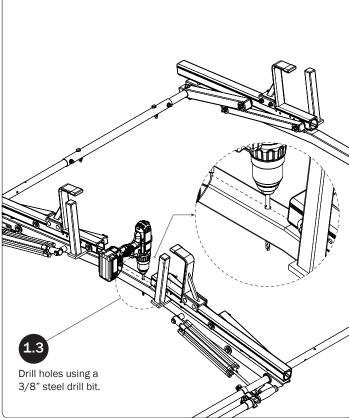
Prior to drilling, mark a center line along the length of the Crossbar to ensure the holes are correctly centered.
