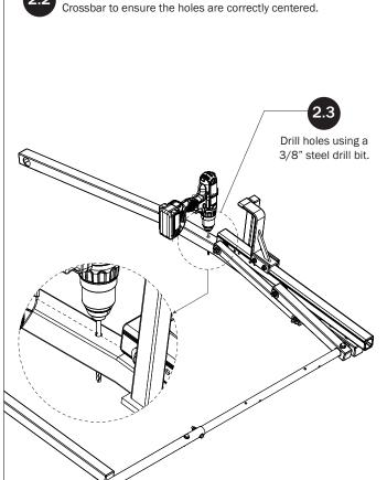
Prior to drilling, mark a center line along the length of the
